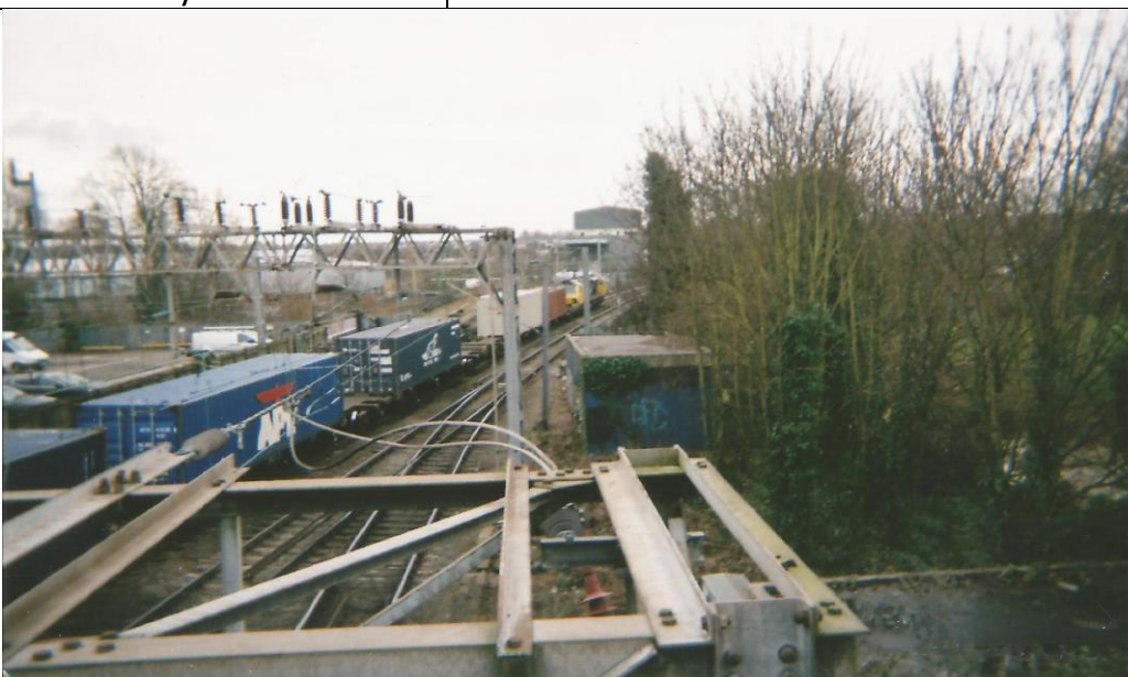
Caption Above: A freight train trundles through the aesthetically new Northampton Castle Station. A single line connects the Brackmills Branch – the stub of the former Northampton-Bedford railway course – to the Northampton Loop which is the slow track part of the four track West Coast Main Line (WCML) which for historical reasons becomes a twin track bypassing Northampton at Blisworth to the west of the urban town. The Northampton Loop carries large amounts of freight as well as the London Midland high frequency passenger operations. Rival train operators are constrained on capacity issues, enter our railway!
